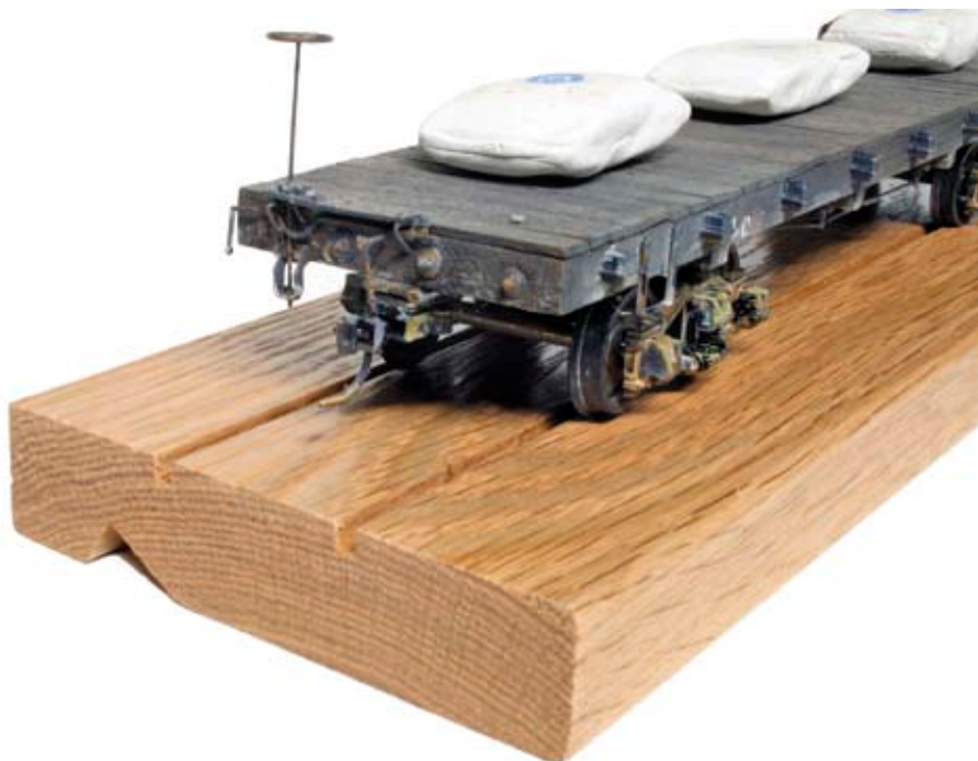
A closeup indicates how easy it is to mount equipment on the shelf. The rear wheels are in the groove, the front ones out. To move them into the grooves, just slide them over until they fall in: much easier than railing stock on track, since you don't have to lift the wheels over the rails.
